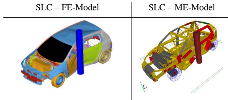
Figure 1: Finite Element and Macro Element Model
